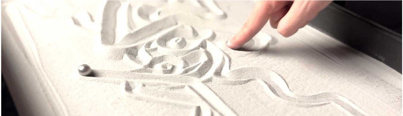
Figure 1: A user is drawing on the sand playground, and the metal ball draws synchronously.
